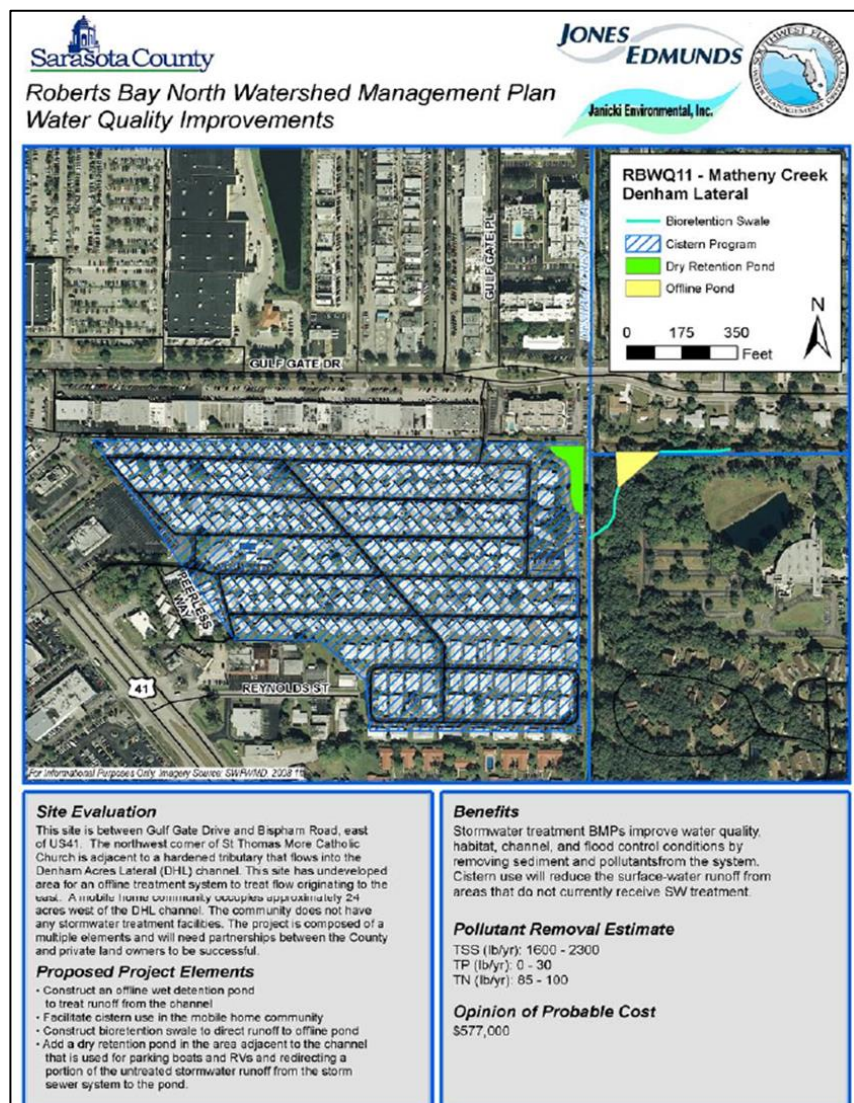
Figure 8 – Overall site plan and potential benefits of proposed Matheny Creek stormwater retrofit project
